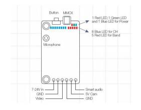
This picture shows a simplified schematic for the circuit board which is used showing the MMCX connection which his used to connect the antenna and then the wires are simply soldered on to the holes at the bottom which is then wired up to the corresponding points on the FC.
