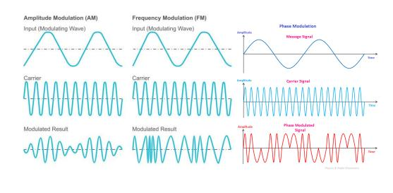
The picture shows the way in which the carrier waves are affected by the inputs in both AM and FM and also phase modulation.
