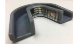
Mouth Guard Biosensor 3D Printed with fully printed electronics and sensors
