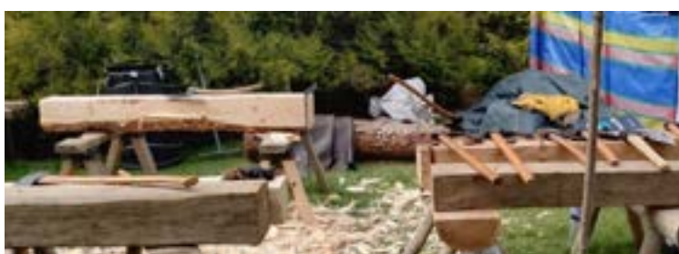
A hewn beam on the left, with a selection of hewing axes resting on other hewn beams on the right.
